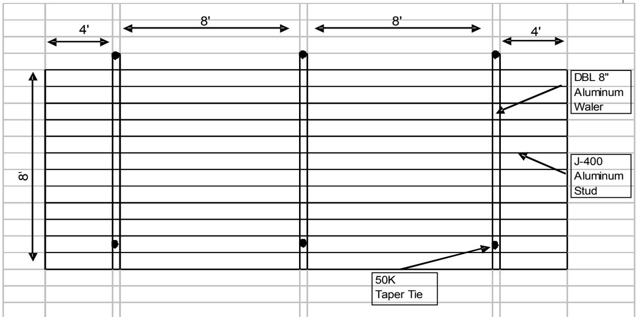
Let's walk through an example of calculating tie lengths on battered walls. Using the equation:
