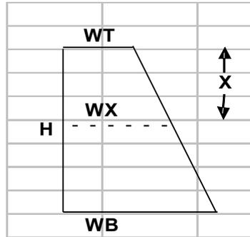
$$\begin{aligned} X &= 5'-0'' \\ \text{WX} &= 12 + 60 \left| \frac{24-12}{120} \right. \\ \text{WX} &= 18'' \end{aligned}$$
